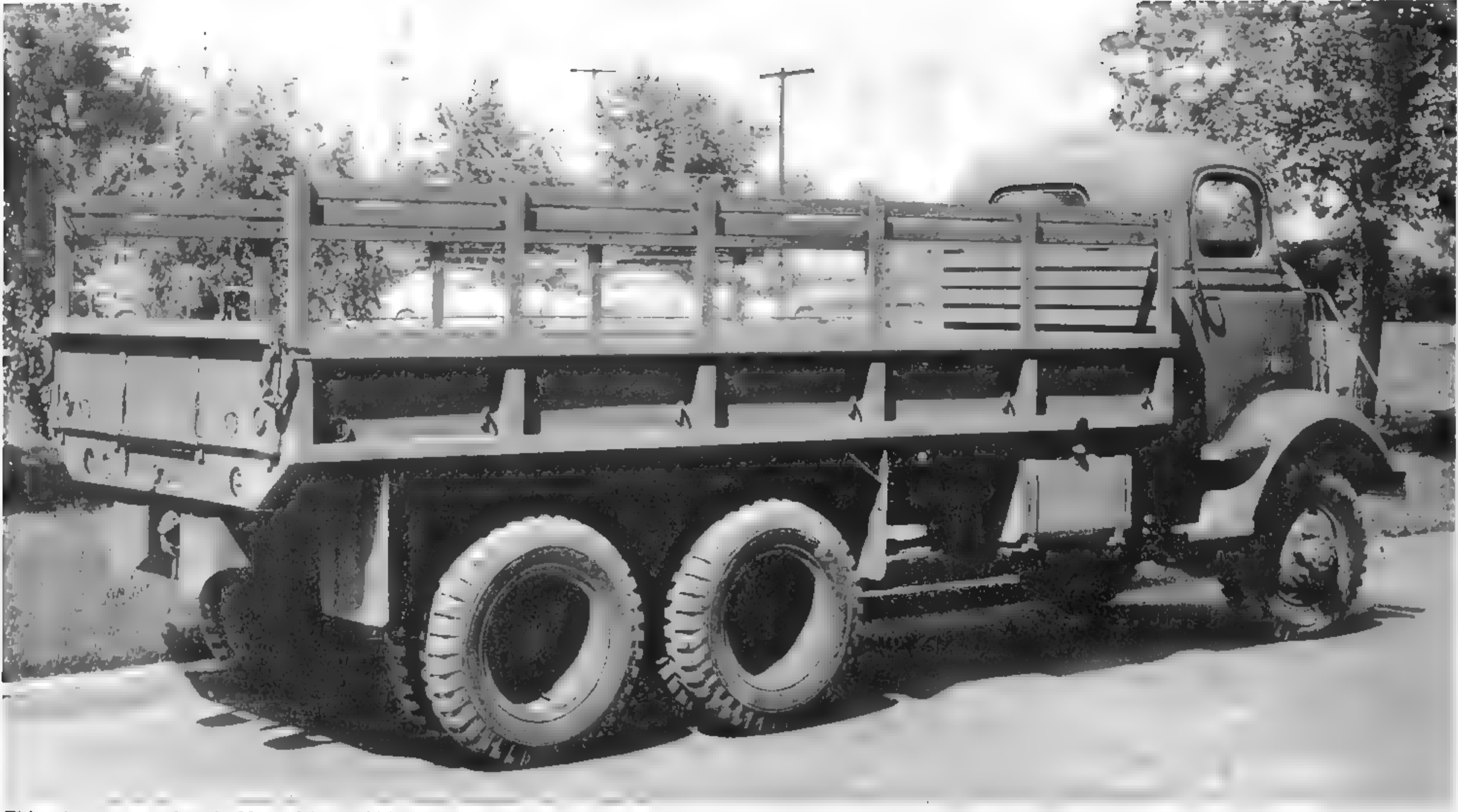
This photo was taken in May of 1942. Although not shown in these photos, a canvas bed cover could be fitted to protect the AFKWX-353 cargo. The cab did not tilt. Engine maintenance was quiet laborious, requiring the removal of much sheet metal. (Photo from Bryce Sunderlin collection)
